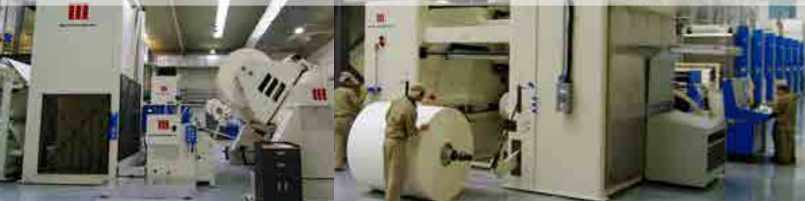
"Martin Automatic MTB butt splicing unwinds at Greatview Aseptic Packaging's new plant at Helingeer, Inner Mongolia. The two printing presses are also equipped with Martin nonstop rewinders for continuous roll-to-roll production."
